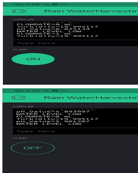
Figure 4: Snapshots of result obtained on Blynk app
