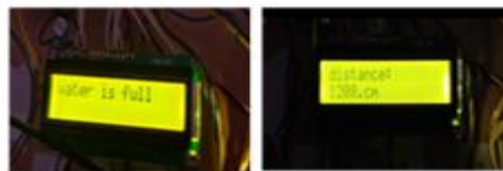
Fig. 5: Output of Ultrasonic Sensor when water is full
