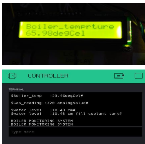
Fig. 8: Display of Boiler temperature, when it increases beyond the Threshold value (LCD and blink app) simultaneously.
