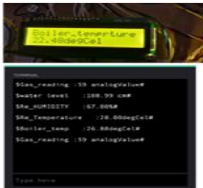
Fig. 7: Rise in temperature of the boiler is displayed both in LCD and blink app simultaneously and continuously
