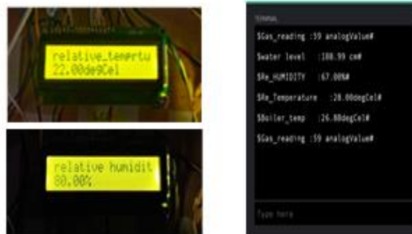
Fig. 9: Relative Temperature and Humidity across the boiler power plant
