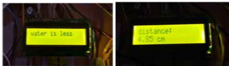
Fig. 4: Output of Ultrasonic Sensor when water is less
