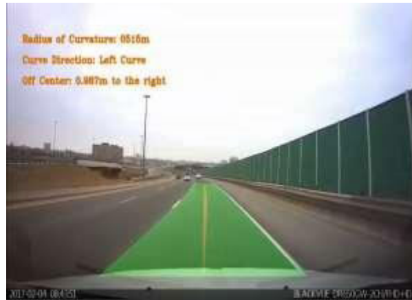
Fig 12. The curve direction is identified as left and the highlighted section indicates the lane that the target vehicle should follow
