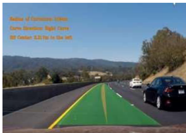
Fig 13. The curve direction is identified as right, and the highlighted section indicates the lane that the target vehicle should follow
