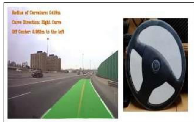
Fig 16. The right curve is being identified and the steering wheel responds correspondingly (towards the right).
