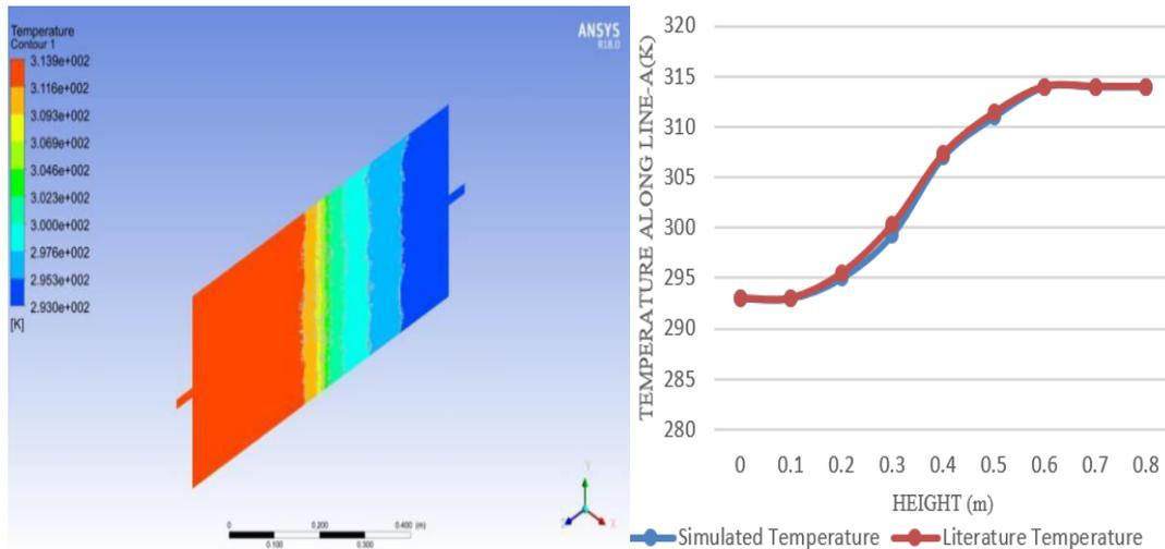
Figure 6. Temperature Contour at Mid-plane of Storage Tank by the end of 1500 seconds
