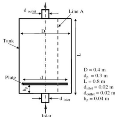
Figure 4. Geometry of the stratification tank
