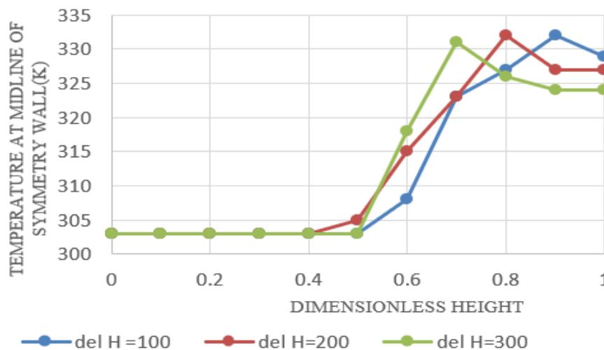
**Figure 19.** Variation of the average temperature of the fluid against the dimensionless height for varied port locations of 100mm, 200mm, and 300mm for respective boundaries
