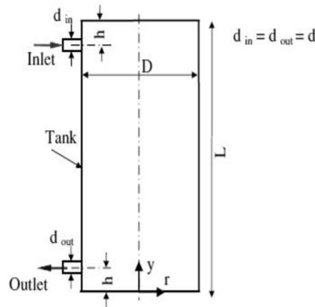
Figure 1. Geometry of the tank
