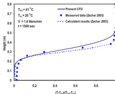
Figure 5. Temperature along with the height of storage tank
