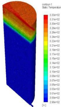
**Figure 21.** Temperature contour at 500 seconds for 0.15kg/s
