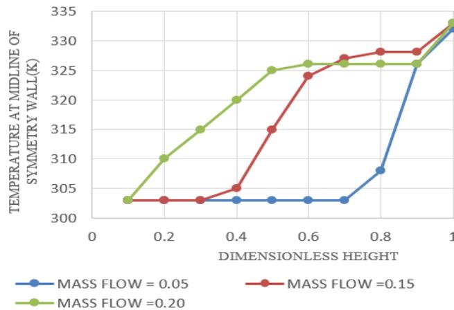
**Figure 23.** Midline Temperature at Symmetry wall Vs Dimensionless Height for different flow rates
