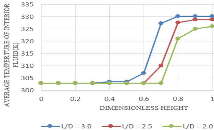
Figure 11. Variation of the average temperature of the fluid against the dimensionless height
