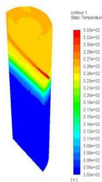
**Figure 18.** Temperature Contour at 500 seconds for 300 mm from the top and bottom of the tank's inlet and exit ports.
