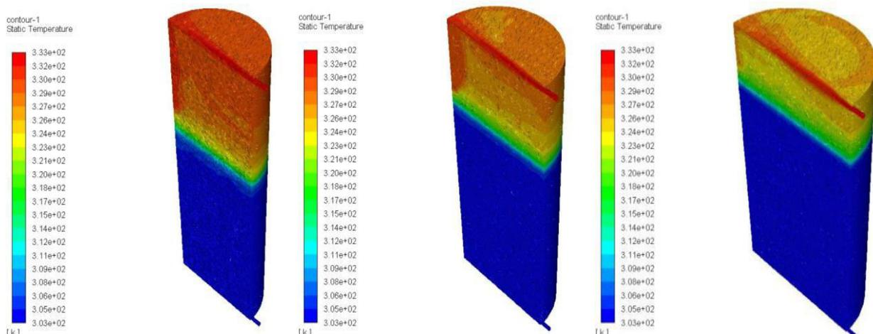
Figure 8, 9 &10. Temperature contour at 500 Seconds for L/D ratio of 3.0 , 2.5 and 2.0
