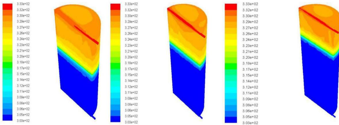
Figure 12, 13 & 14. Temperature contour at 500 seconds for L/D ratio of 2.0, 2.5 and 3.0
