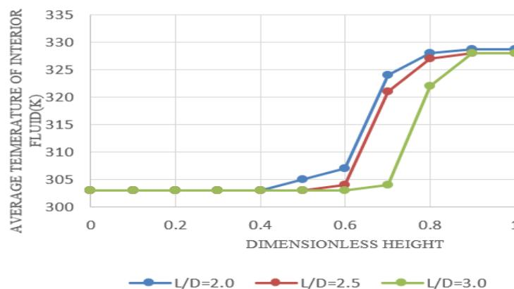
Figure 15. Variation of the average temperature of the fluid against the dimensionless height
