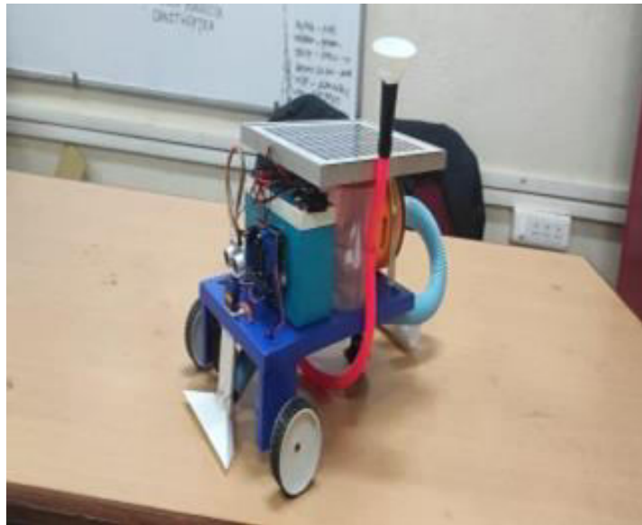
Fig 18: Prototype model of solar floor cleaner robot (side view)
