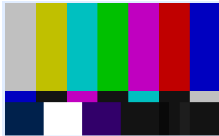
Figure 13 Resultant Color Bar in Response to Timing, Hsync and Vsync
